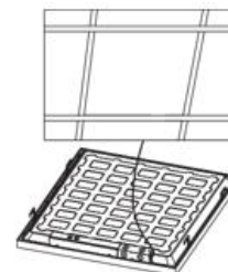
② Feed the main AC wire in driver terminal block respectively, connect the panel light and driver.
